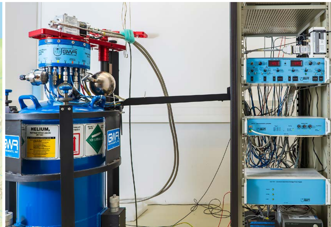
Superconducting gravimeter GWR OSG
