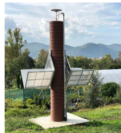
Collocation station with GNSS and artificial corner reflectors.
