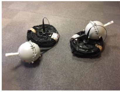
Temperature-measuring surface drifters. Credit: NCE
